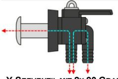
**Y-SEEVENTIL MIT 2x 90 GRAD SCHLAUCHTÜLE UND BORDDURCHLASS (VERSENKT ODER PILZKOPF)**
