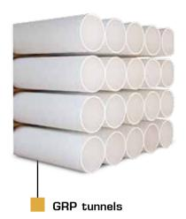
Manufactured from fully isophtalic resin and pre-gel coated, Max Power's high quality tunnels have the added advantage of a first coat of matt before being filament wound. Cutting and drilling can therefore be carried out without the risk of damaging the gel coat on the inside surface of the tunnel.
