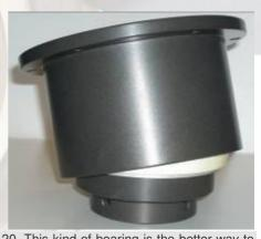
rudder shafts with diameter from mm 50 up to mm 120. This kind of bearing is the better way to fit sloping rudder shafts, because of his self-aligning system (max angle – 18°), the flange remains always flat, avoiding to built recesses or steps on the deck for the vertical alignment between the rudder shaft and the bearing.
