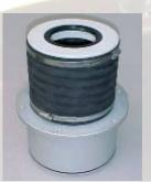
with a self-supporting neoprene tube (height on demand) locked by stainless steel clamps. A ring with gasket is locked on the top of the tube by using stainless steel clamps.
