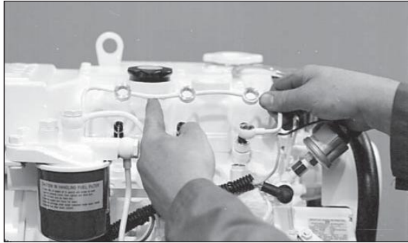
Figure 17: Remove return line.
