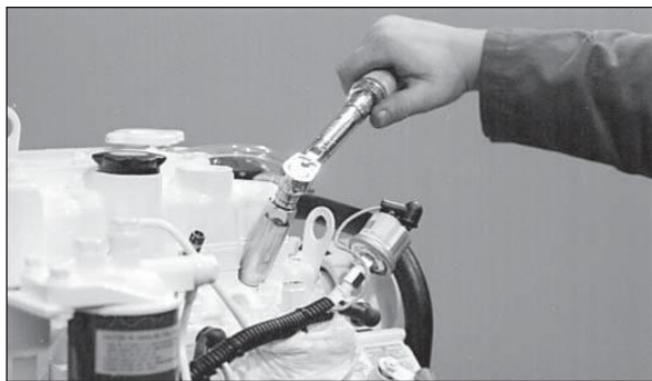
Figure 20: Reinstall injector. Torque to proper tightness.
