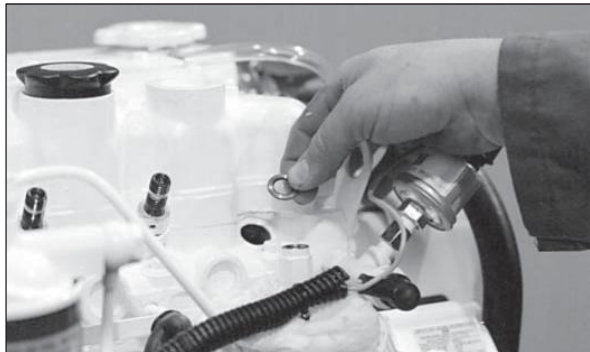
Figure 19: Remove and replace copper sealing washer.
