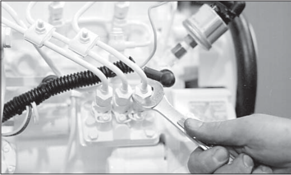
Figure 13: Remove delivery line flare nuts.
