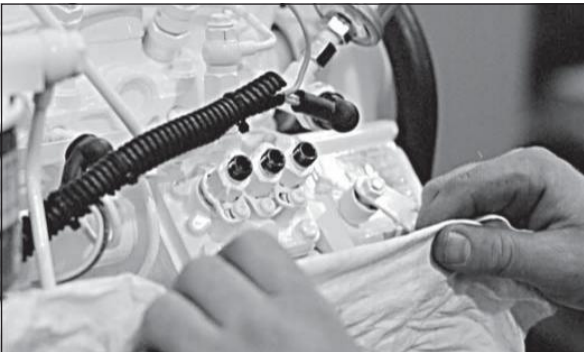
Figure 15: Cover lines, inlets and injection pump outlets.
