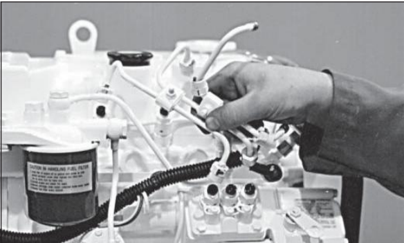
Figure 14: Remove delivery lines.
