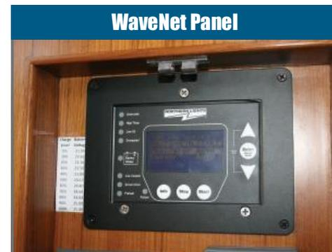
WaveNet can be connected to the pilot house through the NMEA 2000 network for seamless integration with your other marine systems.
