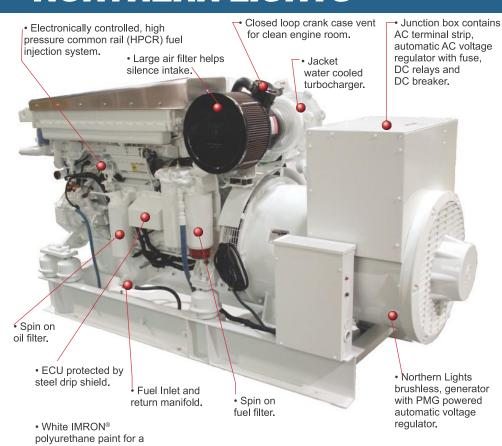
AC Output<sup>1</sup> 250 kW 60 Hz, 1800 RPM 200 kW 50 Hz, 1500 RPM Voltage Regulation ±0.5% Frequency droop control Isochronous 0% Phase and power factor 3 phase-0.8 power factor
