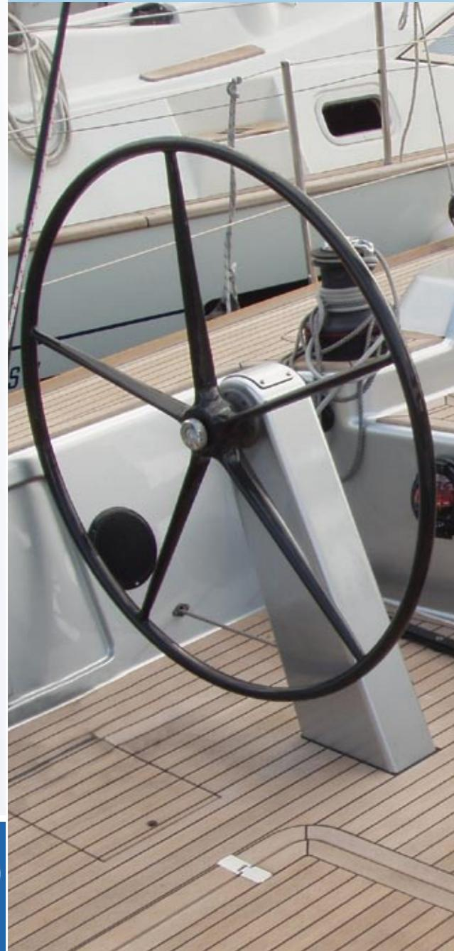
A linear and neat design for this pedestal with a shape lightly trapezoidal that amplifies the effect on the deck and transmit a sensation of strength. The model 609B must be laminated at the deck during the construction to become a sole body with the rest of the boat.
