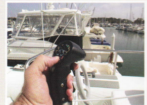
Easy to use proportional controls on all cranes above 1500 lbs (680 kg)
