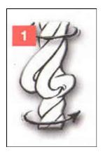
Don't cripple the rope when opening the lay.
