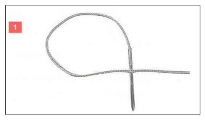
Multiply the diameter of the rope by 50 and mark this measurement from the end of the rope, leave a gap for twice the required eye size and insert the fid and pull end of rope through until it reaches the mark.
