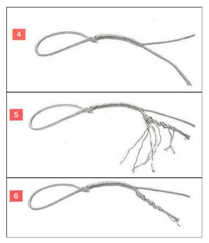
From the tail end of the rope, mark six successive plaits in one direction and a further six successive plaits in the opposite direction. These can then be pulled out and cut at its successive mark.
