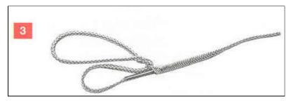
Lay loose end alongside main rope and make a mark approx. 8cm from end of tail. Insert loose end into splicing fid and insert fid at the last tuck and push through the centre of the rope, to emerge at your mark.
