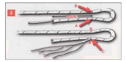
Measure 30cm from end of cover and mark 'A'. Form eye size and mark 'B' on standing part of rope. Open cover at 'A' with a fid and take out core, marking it 'C' at hole. Taper core over approx. 20cm from 'C', removing 6 individual strands.
