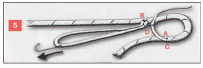
Mark 'C' should meet with 'D' and tail should disappear inside core loop.
