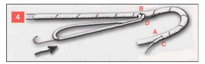
Insert large needle into core at end of loop, bringing eye out at 'D'. Thread core tail into needle and pull back out.
