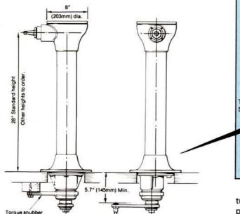
A totally new design based on the 'Cobra' concept, incorporating an additional ultra-compact gear reducer at the base of the pedestal to provide a superb system for yachts up to 60' L.O.A.
