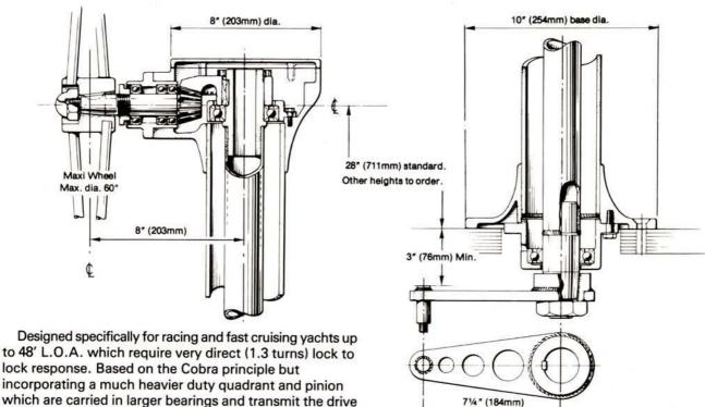
lock response. Based on the Cobra principle but incorporating a much heavier duty quadrant and pinion which are carried in larger bearings and transmit the drive through a larger dia. down tube, to handle the greater torques generated. King Cobra retains the same advantages of the Cobra
