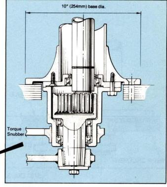
Available in two versions; the standard unit gives 3 1/3 turns of the wheel for full rudder travel and is aimed primarily at the larger cruising yacht.
