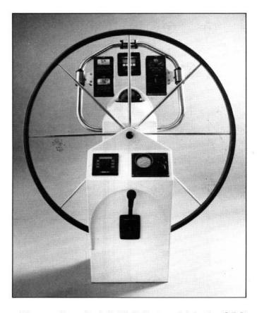
The space frame is clad with high strength injection G.R.P. moulded panels for style and durability. Practically however they are rapidly removable to gain access to the steering and autopilot mechanism for installation and servicing. A wiring loom for the instrumentation is fed through the pedestal and is immediately accessible.
