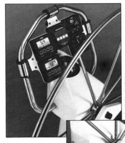
Instruments mountings are fully articulated and can be adjusted for port or starboard viewing.
