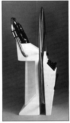
I.S.S.TM is more than a new yacht pedestal it offers for the first time the facility to mount instruments, engine controls, navigational aids and the autopilot on one pedestal. Uniquely the autopilot drive has been incorporated into the pedestal space frame. When disengaged, there is zero drag on the steering system.
