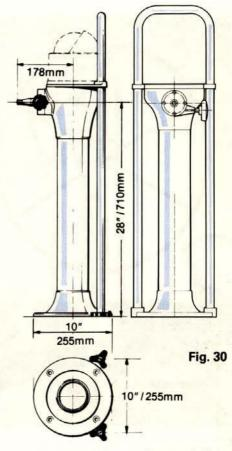
Pedestal with retrofit guardrail. (Fig 30 Page 47)
